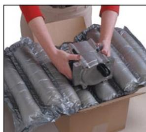
3. The operator centres the product on the tubes, setting both into the carton.
